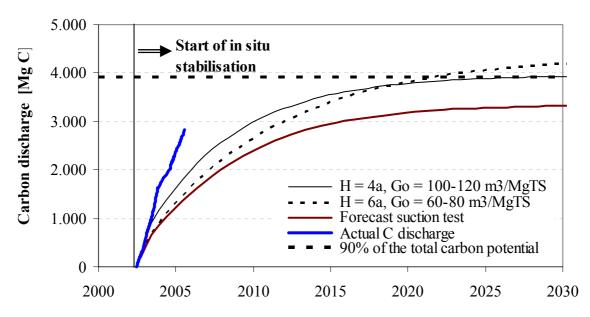
Figure 4: Range of the biologically convertible carbon, dischargeable via the gas path, under anaerobic milieu conditions from 2002 onwards. Comparison with the actual carbon discharge as a result of aerobic in situ stabilisation
