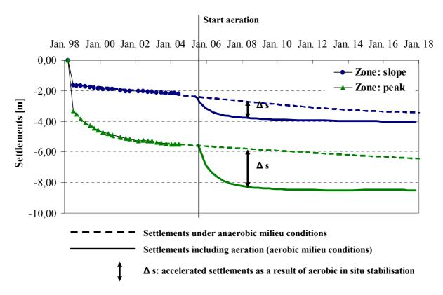
Figure 2: Course of the settlements in the proximity of two gas wells in the peak and slope area under anaerobic and aerobic milieu conditions
